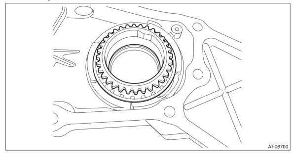
8) Remove the oil seal from the oil pump chain cover.
