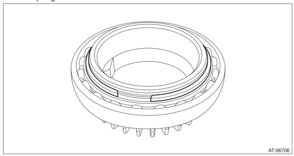
2) Remove the ball bearing using ST. ST1 498077600 REMOVER ST2 399513600 INSTALLER
